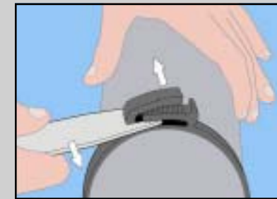
4. To remove the clip, place the HCL removal tool at the bottom part of the female jaw and slide or twist sideways.
