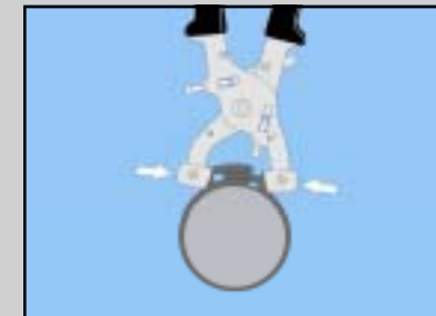
3. Using the HCL hand tool or pliers, simply squeeze the jaws together until a secure fit is achieved.
